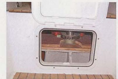
Access to steering cables through the trapdoor on the transom extension
